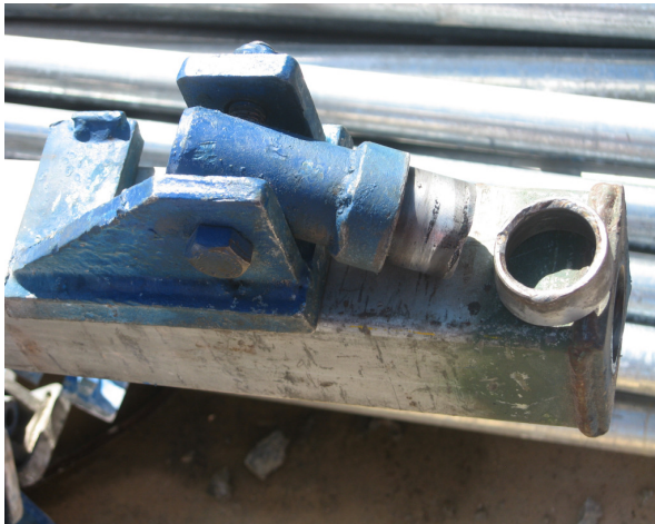
View of failure of weld on prop foot
